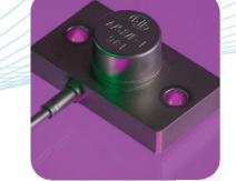
High output industrial grade accelerometer with integral hard-line cable, and available in two temperature ratings. Hermetic construction is proof against degradation under severe operating conditions including high pressure fluid immersion. /F version is suitable for milli g monitoring with appropriate instrumentation.
