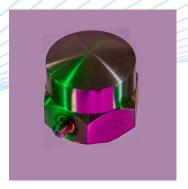
Ultra high output, multiple shear plate voltage accelerometer. Shear plate construction provides near total isolation from mechanical inputs other than acceleration, thus safeguarding measurement integrity in applications where vibration is accompanied by high dynamic strain levels.
